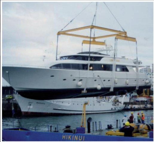
Lifting and transportation of 108-ton Super yacht
